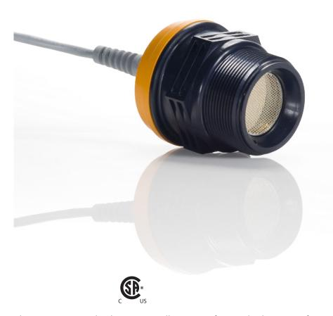
The IRU-9400 series has a versatile range--from 6 inches to 35 feet--and a sensitive electrostatic transducer for detecting difficult targets. This sensor is great for non-reflective and/or soft surfaces. With built-in technology to compensate for temperature changes, the IRU-9400 is well-suited for non-traditional ultrasonic applications and is recommended for indoor or controlled-humidity environment uses only.†
